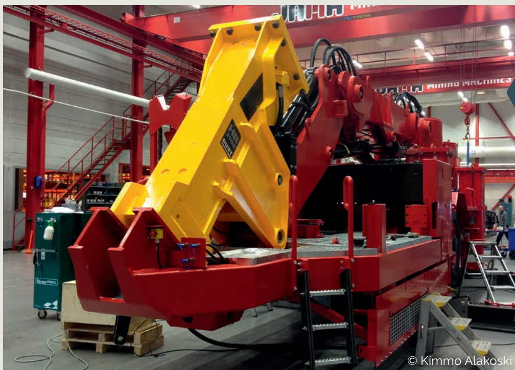
JAMA produces special carriers for scaling and other underground mining applications. The latest new model breaks oversized stones with an Epiroc HB3100 DP breaker in Kiruna Mine in Sweden. This carrier is not self-propelled and it will be moved between the job-sites by an underground loading machine.
