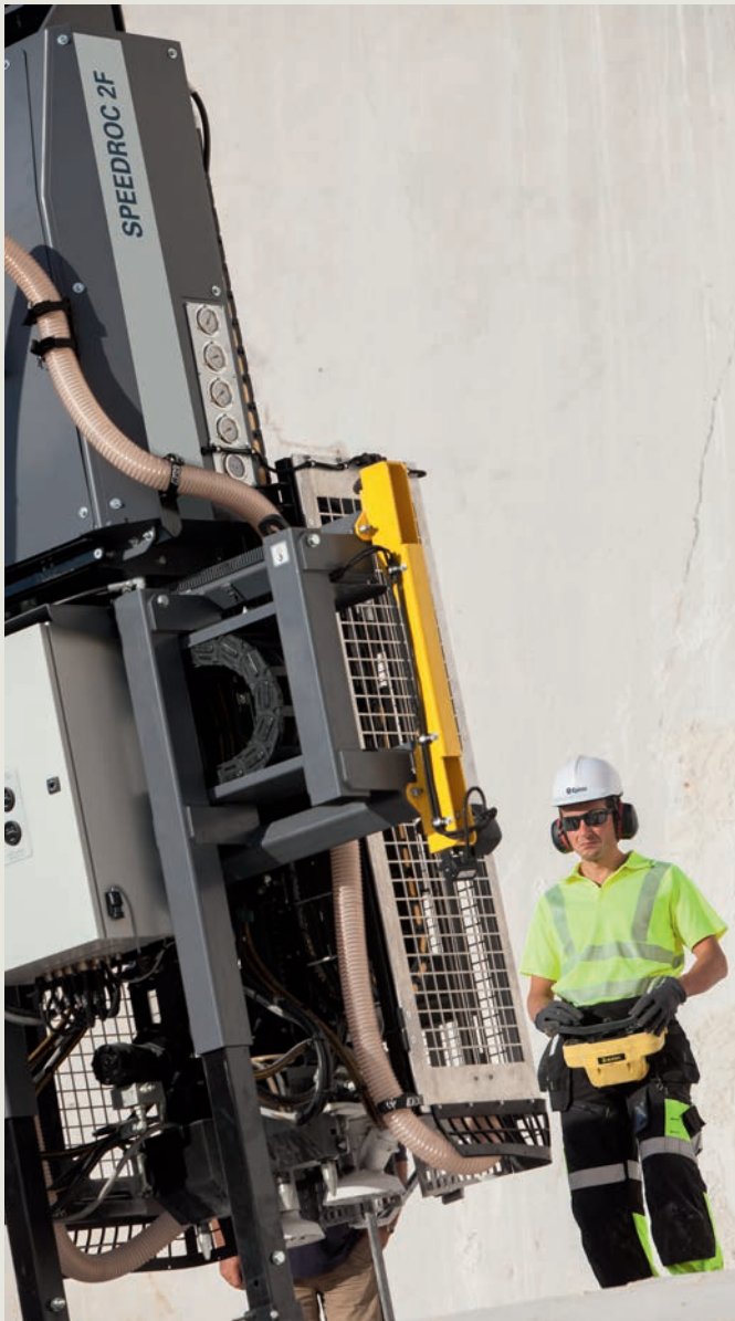
The radio remote controller releases the operator from the cabin to get a better view of the tool.
