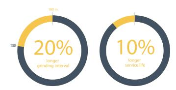
The average grinding interval was almost 20% longer with Powerbit Underground. The bit proved highly effective on mixed rock, performing well in the igneous formations on site. The high flushing capacity was effective on soft clay pockets.
