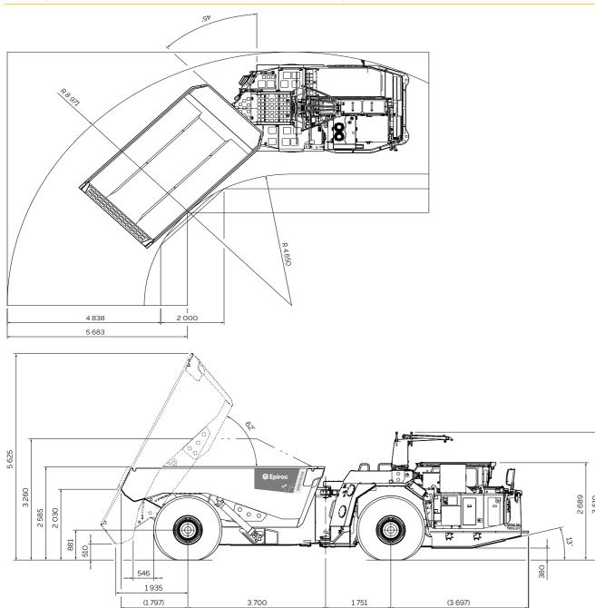
All dimensions are shown in millimeters (mm). Dimensions and calculations shown are based on standard vehicle configuration with 30 mm tire deflection, unloaded.
