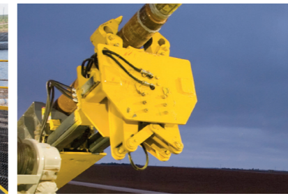
The Driller has complete control over the connection process by clamping and extending the drill pipe to the top drive and threading it into the pipe for a secure connection before bringing the drill pipe in through the drill floor.
