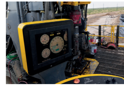
A robust, military-grade control console monitor displays drilling parameter gauges, engine parameters and drilling system diagnostics.
