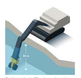
Can be used up to 30 meters underwater without additional installation or modification.
