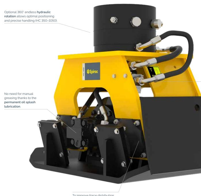
To improve force distribution and thus lessen the strain, the outward shock mounts are tilted 15°.
