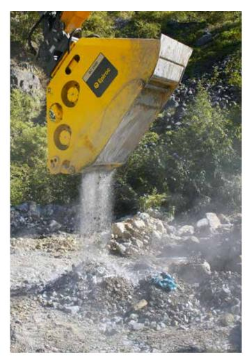
Our Bucket Crushers combine low maintenance and high performance. On-site crushing also means less transportation and dumpsite costs.
