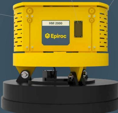
Built-in **generator with advanced control technology** provides faster material pick-up by a quick magnetization with impulse excitation and material release by automatic demagnetization with counter voltage and sequence pulsation.
