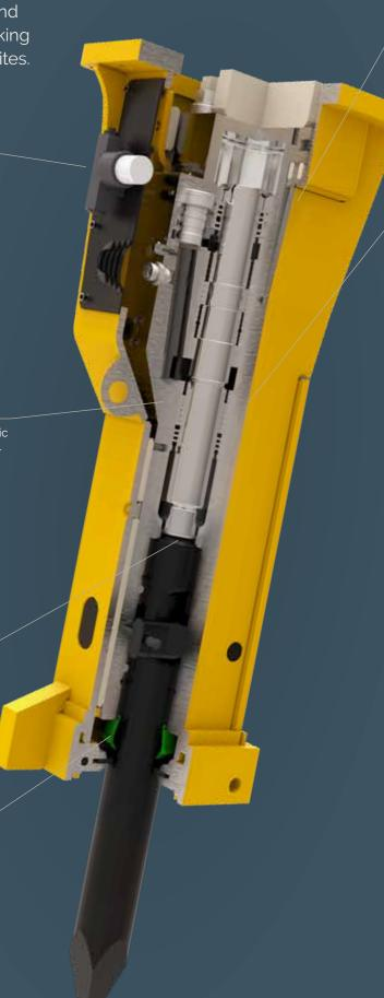
The piston stroke length system **AutoControl** automatically adjusts the output balance during operation thus optimizing performance.
