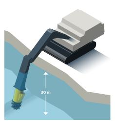
Can be used up to 30 meters underwater without additional installation or modification.
