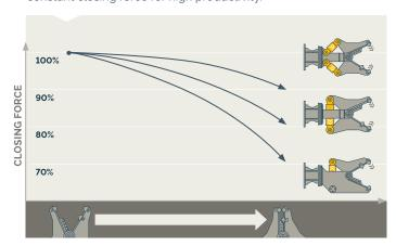
Two independently moving jaws eliminate displacement force, thus lowering stress levels.
