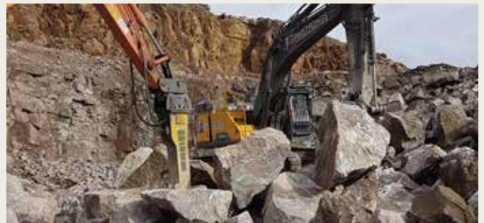
MB 1650 on 21t excavator breaking oversized granite boulders on the rock pile
