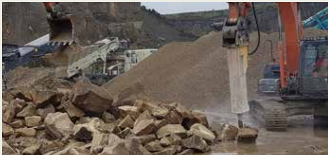
MB 1650 on the 21t excavator in the dedicated area for secondary breaking near to the crusher and screener station
