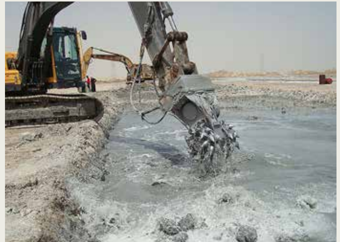
Salt mining with ER 1500X in Saudi Arabia
