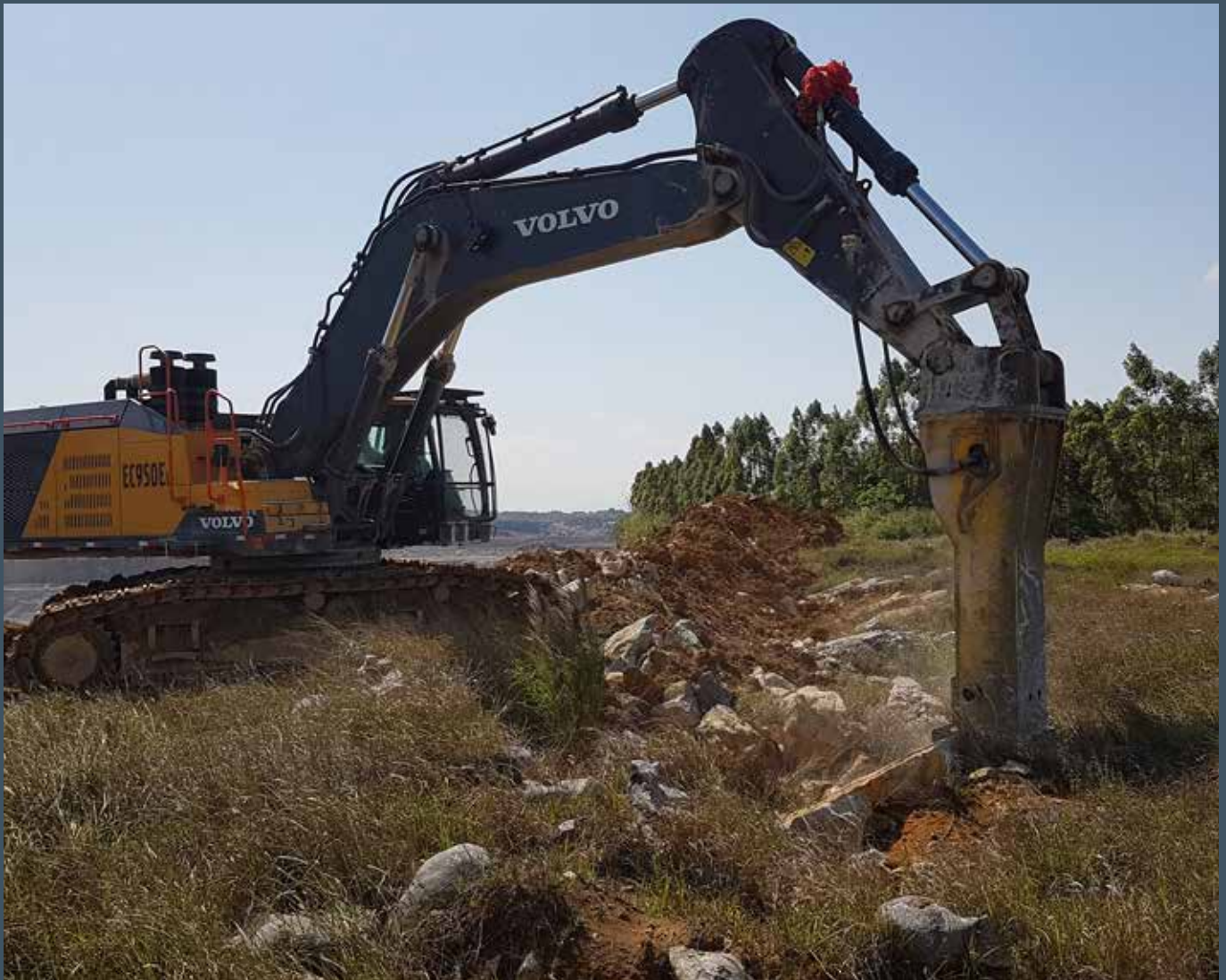
HB 10000 on a 92t excavator breaking limestone boulders in the overburden
