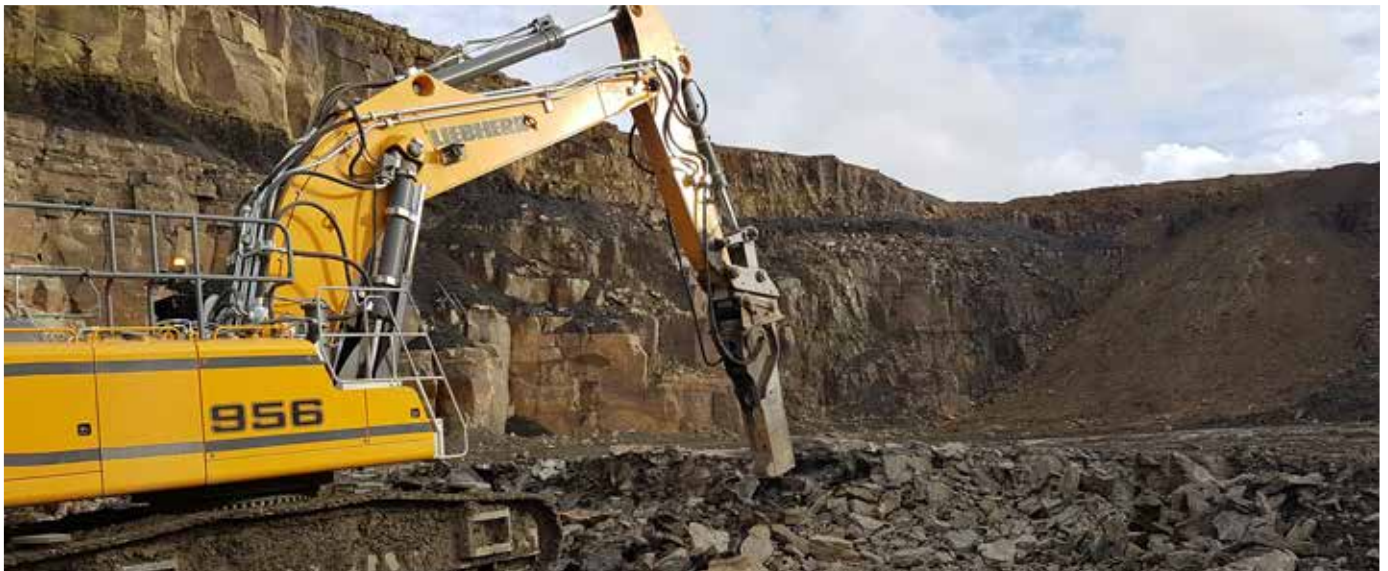
HB 4100 in selective excavation of low quality rock layer from a sandstone deposit in England
