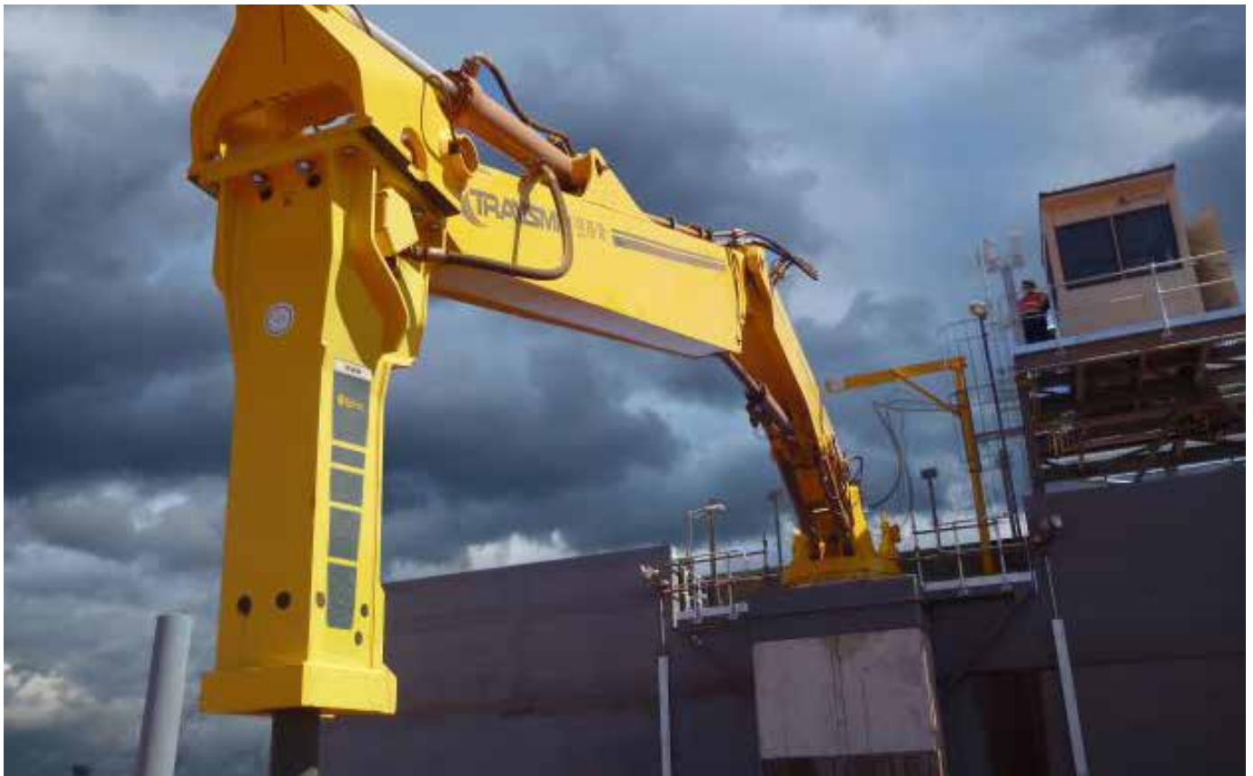
HB 2000 on a pedestal boom at the crusher station
