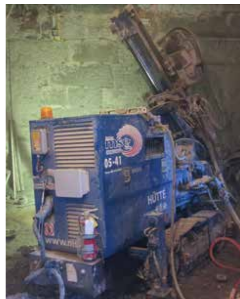
The Hütte HBR 202 E can tram through doorways less than a meter wide and squeeze into tightly confined areas as in this corner. Confined spaces present no extraordinary ventilation concerns, as the rig neither consumes oxygen nor emits exhaust.
