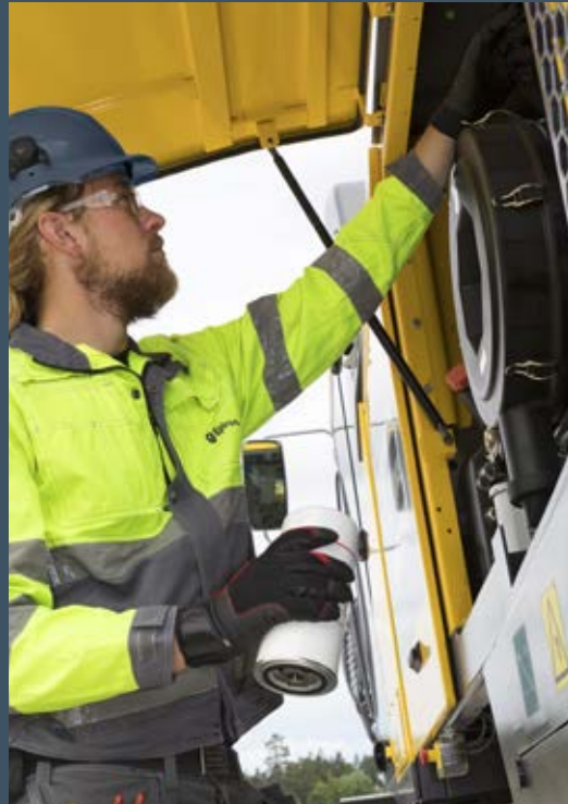
Figure 1: Easy access to service parts at eye-level, from a secure position, is crucial in drill rig design, not least for reaching parts that may need frequent attention such as filters.
