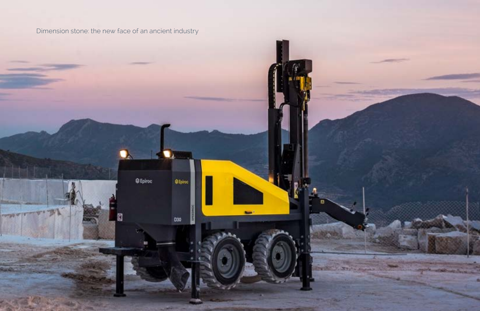
The SpeedROC D30 drilling a pilot hole for diamond wire cutting.
