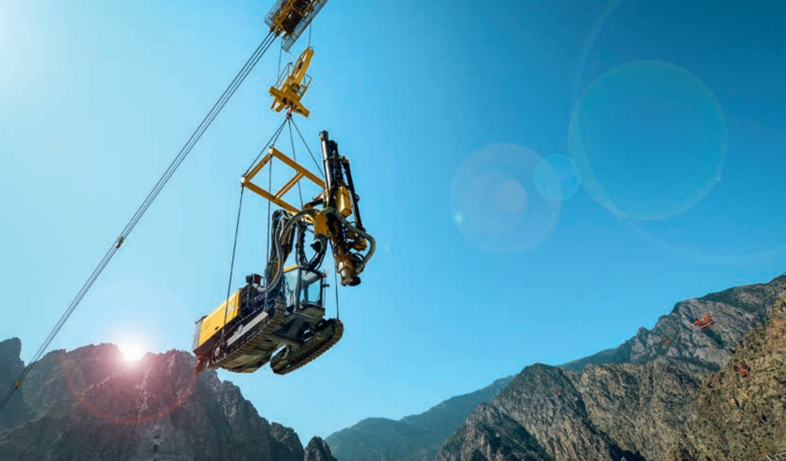
Innovation is key in challenging projects. A cableway was built to get the equipment in place.
