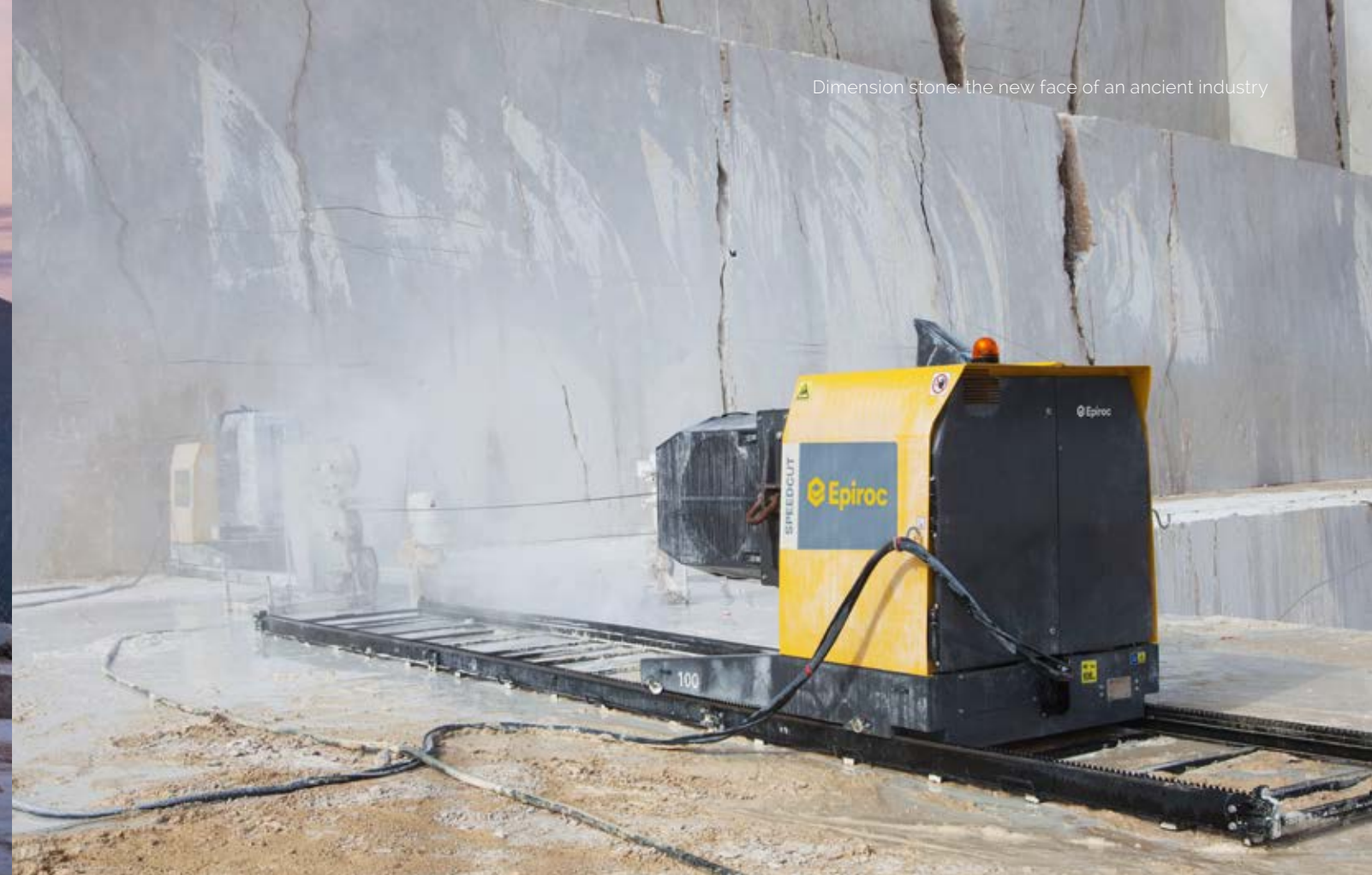
The SpeedCut 100 with a wire speed of up to 45 m/s.
