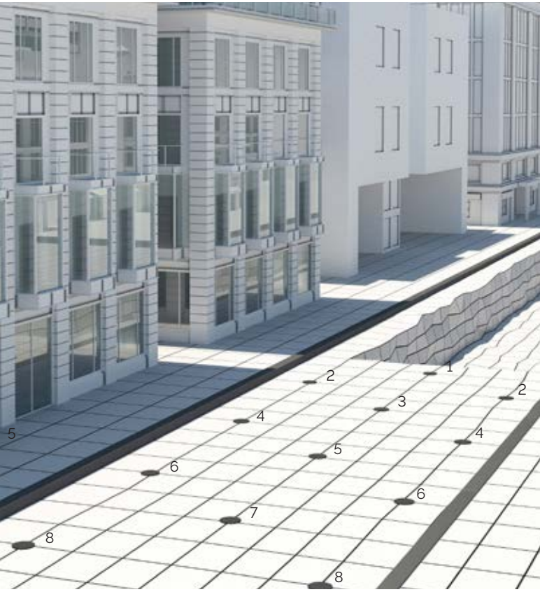
Figure 3: Small diameter blasting in urban areas using 30–45 mm holes.
