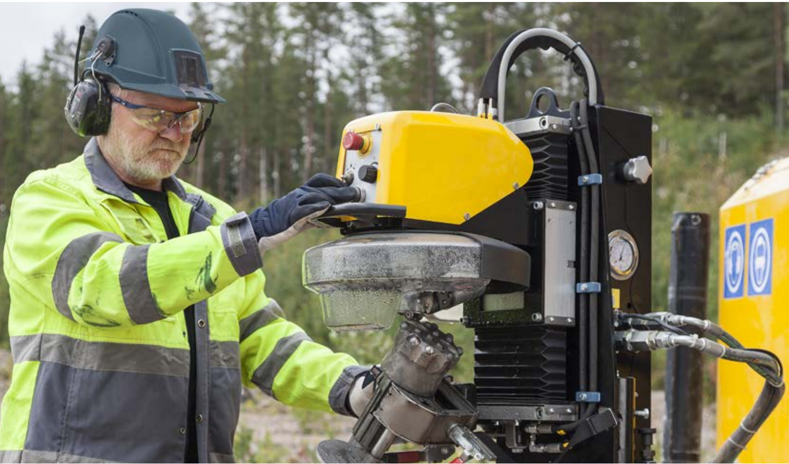
Bit grinding in the field with a Grind Matic RH3.
