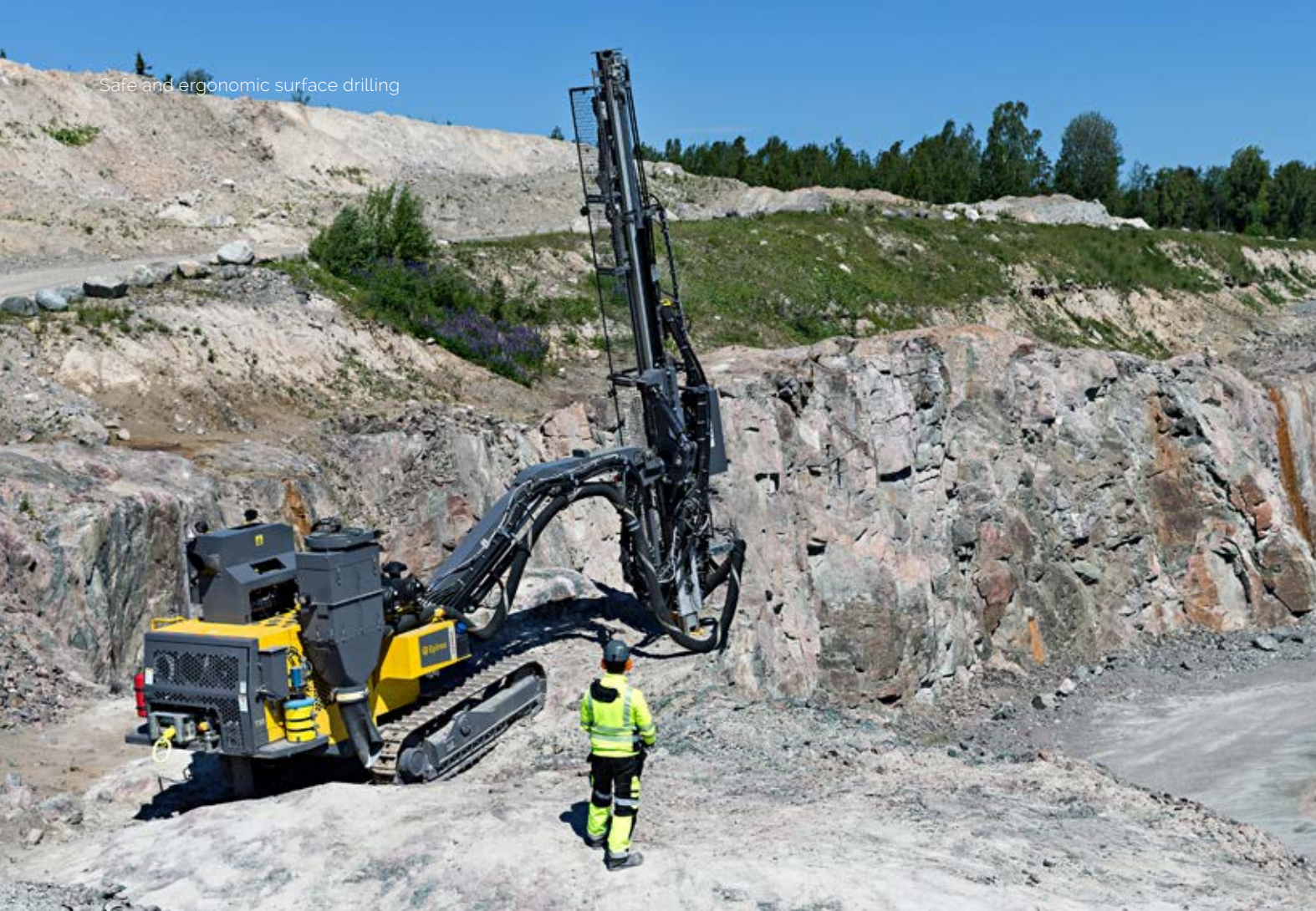
Figure 4: Safe tramming over uneven ground with an oscillating undercarriage.
