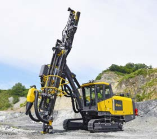
The PowerROC T45 is modular designed with a low number of moving parts.
