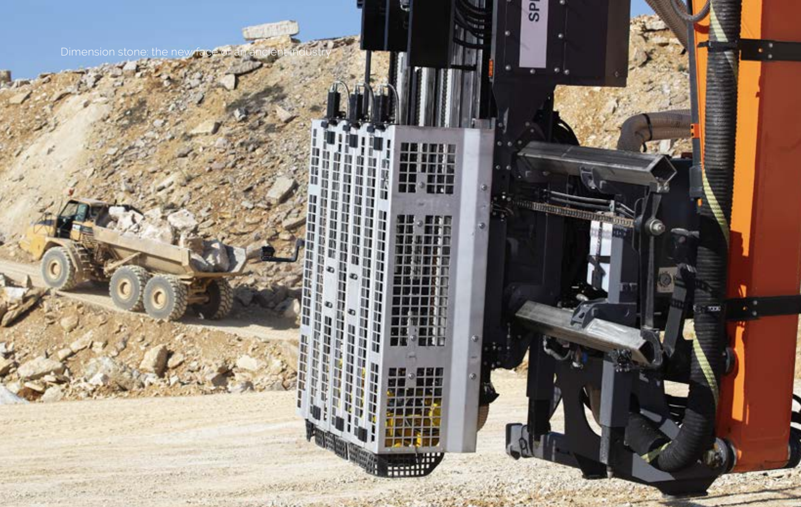
The SpeedROC 3F with three feeds and a protective guard.
