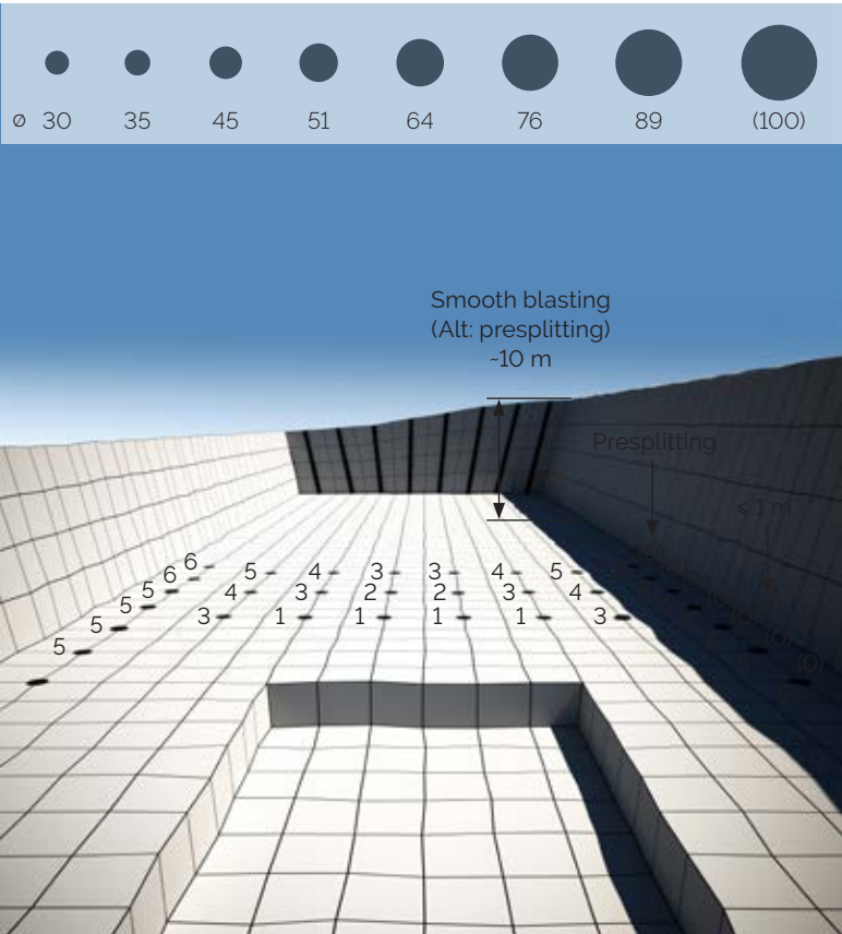
Figure 4: Trenching for pipelines outside urban areas using 51–89 mm holes.
