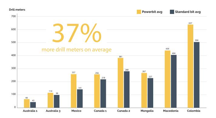
Test results show that Powerbit Underground provides 37 percent more drill metres on average before bit discard than a standard drill bit. The chart shows the location of the test mines used for testing.
