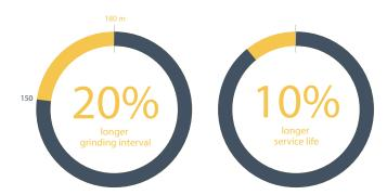
The average grinding interval was almost 20% longer with Powerbit Underground. The bit proved highly effective on mixed rock, performing well in the igneous formations on site. The high flushing capacity was effective on soft clay pockets.
