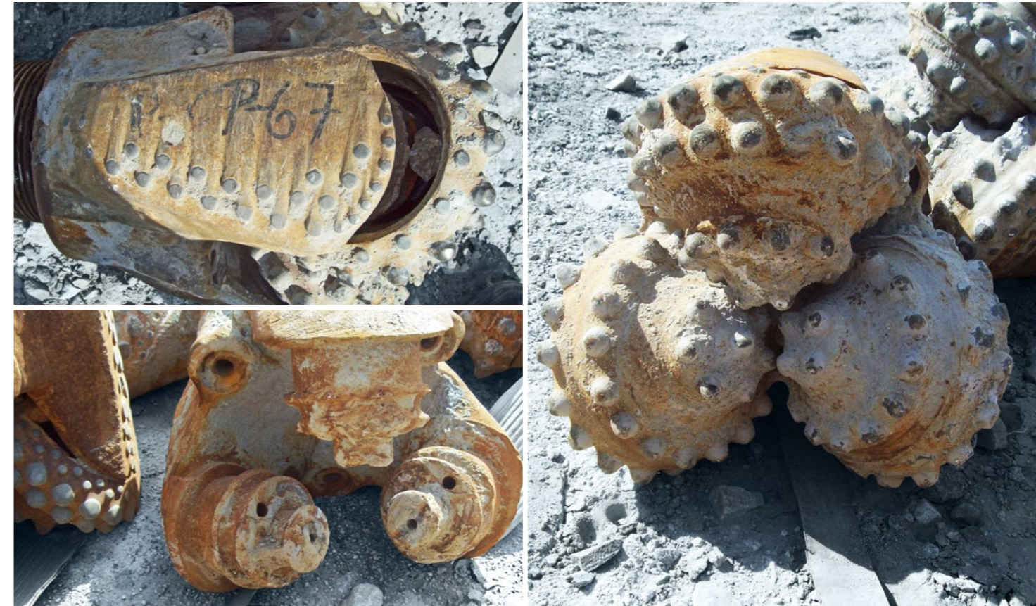
These bits are too worn out to be effective anymore.
