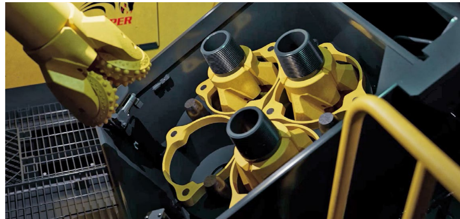
Epiroc high performance bits on the ABC, waiting for the turn.
