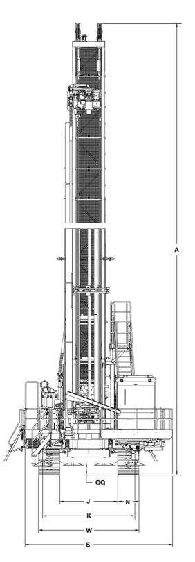
Approximate shipping dimensions for crated PV-271 with 55 ft tower (actual dimensions will vary based on rig configuration).
