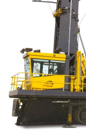
Robust "live tower" design can be raised and lowered with a full carousel and the rotary head at the top of the tower. State-of-the-art tower construction is designed to last for the entire life of the machine.
