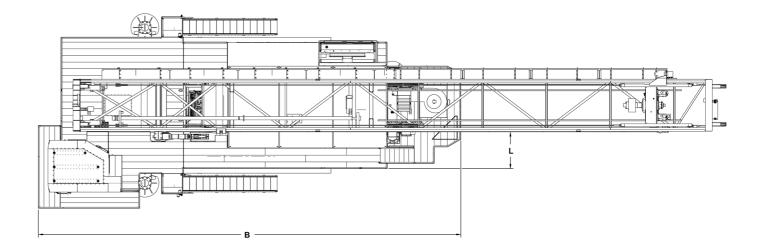
'Approximate shipping dimensions for crated PV-351 (actual dimensions will vary based on rig configuration). ''Fall off will vary greatly by machine and options.
