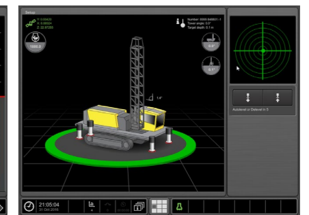
Setup and Propel: shows machine conditions during setup and while propelling.
