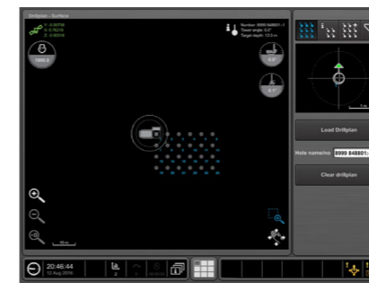
Drill Plan: shows the interactive drill plan.
