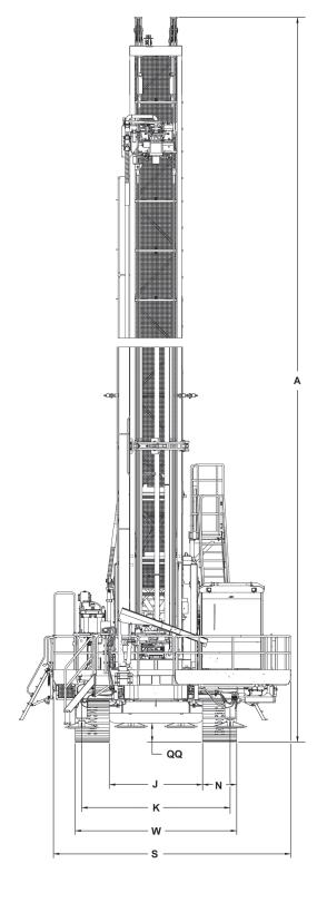
'Approximate shipping dimensions for crated Pit Viper 271 XC (actual dimensions will vary based on rig configuration).
