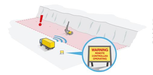
BenchREMOTE can be used up to 100 meters horizontally and 30 meters vertically from the remote rig, Operators can be highly productive without ever having to enter a hazardous area.
