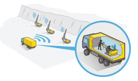
BenchREMOTE can be installed in a customer-supplied vehicle, trailer or container. All BenchREMOTE controls and screens are the same as in the real rig cabin – SmartROC operators will feel right at home.
