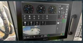
The Rig Control System features an intuitive touchscreen display which presents all the necessary information clearly to the operator and offers assistance during troubleshooting. control and accuracy, COPROD combines the This keeps downtime to a minimum.
