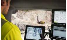
The BenchREMOTE option enables one person to safely control up to three SmartROC automatic rod handling system. The system rigs at the same time from a horisontal distance of 100 meters. This increases operator productivity dramatically and takes safety to a whole new level.
