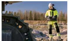
The optional Radio Remote Control allows th operator to step outside the cabin and control a SmartROC D50 from a safe distance when necessary. The integrated display shows all the basic information needed to run the rig.
