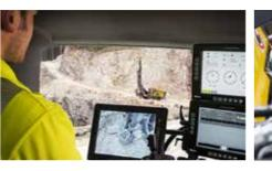
The BenchREMOTE option enables one person to safely control up to three SmartROC automatic rod handling system. The system rigs at the same time from a horizontal distance of 100 meters. This increases operator productivity dramatically and takes feed rate safety to a whole new level.
