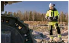
The optional Radio Remote Control allows th operator to step outside the cabin and control a SmartROC D55 from a safe distance when necessary. The integrated display shows all the basic information needed to run the rig.
