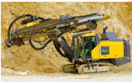
When equipped with the standard feed option, the FlexiROC D60 is capable of handling an even wider range of drilling angles with ease.
