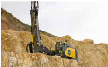
The FlexiROC D60 is built for high efficiency mining. Its DTH hammer benefits from a precisely matched compressor.
