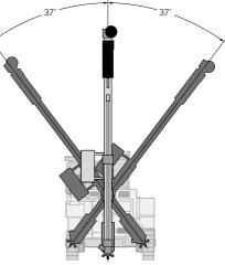
Normal position range in downwards directed drilling (extra long folding boom)
