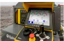
The Christensen 160 Smart control system offers the operator automated drilling. This increases productivity and can dramatically each hole is logged by the system and can be exported into Exploration Manager. This software presents users with the ability to analyze data, find improvements and optimize drilling performance.
