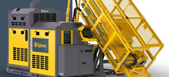
The rods are extracted by the head (pull-by-head) which offers increased automation and safety as well as boosting reliability.
