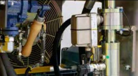
An inductive water flow meter, without moving parts, and a highly accurate pressure sensor increases flushing reliability and availability of the machine.
