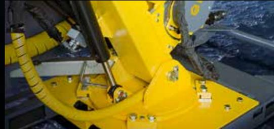
The unique combined turntable and positioning arm fitted to the Diamec PHC 4 and 6 enables easy, fast and accurate set up.
