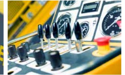
**The pilot hydraulic control system** provides the operator with full control. The operator station works at a reduced hydraulic pressure (max 50 bar) which means it's safer for the operator and lighter in weight.
