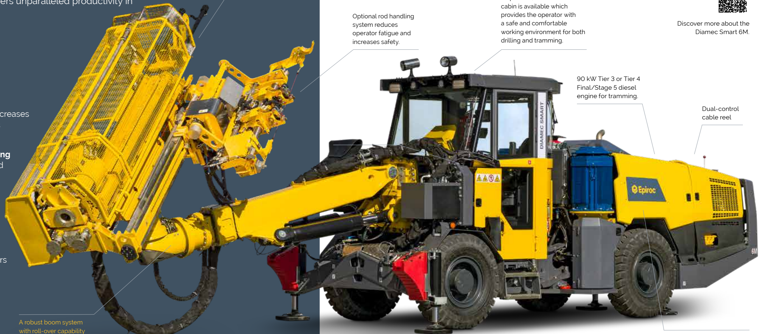
An enclosed canopy helps to reduce noise whilst gullwing doors provide easy access for service and maintenance.
