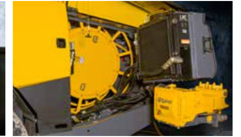
The optional HD oil cooler and Trido pump are both mounted on a swing arm to improve access for servicing.
