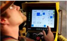
All drilling functions, including the rod handling, are easily performed from the increased safety. If there is a loss of hydraulic light-weight control panel positioned a safe distance away from the rig.
