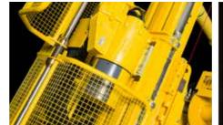
The rotation unit has a sealed gear box, thus lowering operational costs - especially for up-hole drilling.
