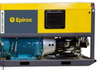
Robust electrically driven power unit with triple hydraulic pumps providing optimized power for the rotation unit and a dedicated pump just for the flush pump.
