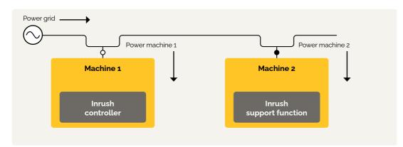
**Inrush**: Controlling this action when connecting and supporting other machines keeps the system stable in weak grids.
