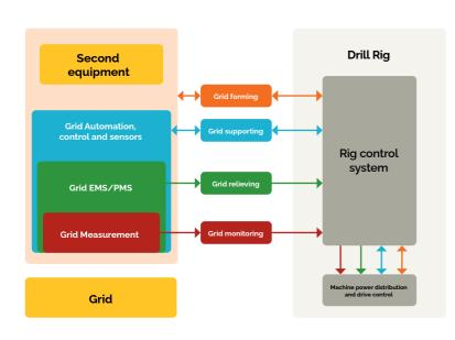
This figure represents different level of communication required for various degree of grid support e.g. monitoring need only grid measurement while grid relieving includes grid measurements and information from energy/ power management system.
