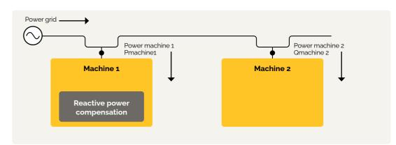
Reactive support: A double win here, as it reduces loss and enhances power capacity.
