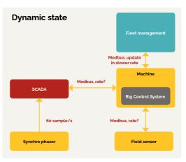
Here, we see the measurement from a remote terminal unit to SCADA and then to the machine control system in steady and dynamic states. While SCADA handles steady-state quantities, retrieving dynamic changes from the grid to the machine through SCADA is harder.
