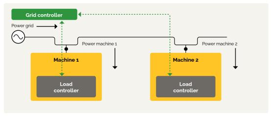
**Load management control:** New load connections are controlled through available generation and spinning reserves.
