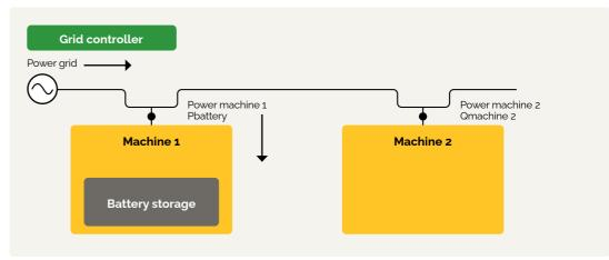
Storage: Using battery storage, we can perform peak shaving during high loading.
