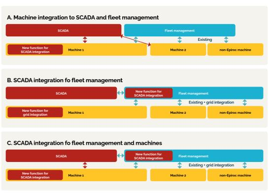
Here, we see an alternative structure for grid integration, in which we gradually move from a more limited integration (A) to a more profound and complete one (C).
