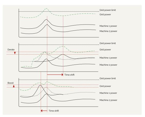
Peak power: By controlling this, it's easier to plan the use of multiple machines.
