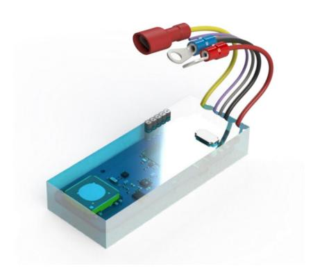
The Pulse130 is a small pedestrian tag designed to fit into most cap lamp brands. The cap lamp is fitted with a sub-GHz RF transceiver and a 125 kHz LF receiver, enabling the tag to detect magnetic fields generated by the Pulse660 and Pulse560. The tag then communicates this information to sensor devices, indicating the pedestrian's location within the zones.
