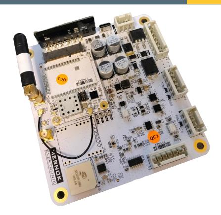
The PulseLink100 is similar to the Pulse660, and also generates a low-frequency magnetic field with object-penetrating capabilities. This magnetic field is created along a flexible cable transmitter, which allows for the generation of longitudinal fields tailored to the operational area. This ensures that the field conforms to the operational area, effectively covering all hazardous zones.
