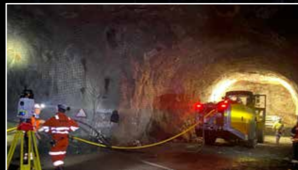
Total station navigation and Simba COPROD drill rig at Pucobre mine.
