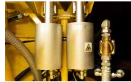
The new additive dosing pump combines the metering system and pump into one, to achieve higher accuracy.
