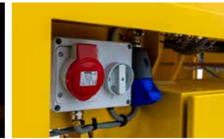
External three-phase and single-phase electrical outlets to facilitate convenient and flexible operations.
