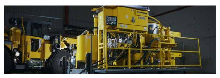
The MWD-data from the face drilling rigs can be automatically transferred to the Unigrout M2 S.
