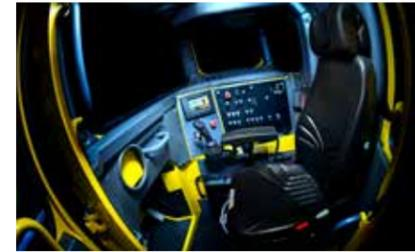
The comfortable and safe cabin is ISO FOPS and ROPS certified and it features a footbox to maximize leg room.
