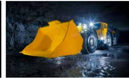
The Scooptram ST18 S is equipped with smart features, including traction control and overspeed protection, and can be used in combination with Deep Automation - Epiroc's cutting-edge set of automation systems and applications.
