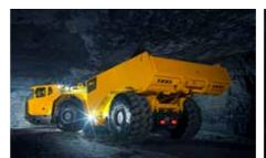
The smart, hydraulically operated tailgate works as a spill guard and supports the filling process with one extra side in the box. this truck easy to operate for long periods.
