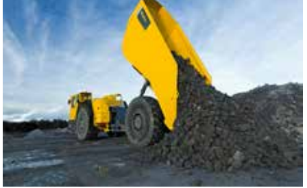
The robust dump box has a load capacity of 66 metric tonnes and the load-weighting system monitors the loading process.
