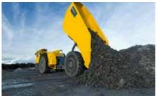
The robust dump box has a load capacity system monitors the loading process.
