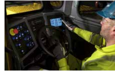
The cabin provides comfort to the operator with its low noise level, air conditioning, spring-suspended and adjustable seat, user-friendly display, and easily accessible controls.
