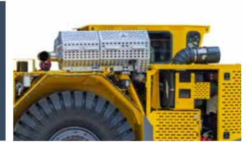
The Minetruck MT2200 Stage IV engine's aftertreatment system is designed to significantly reduce toxic gases, including particulate matter (PM), nitrogen oxides (NOx), and hydrocarbons (HC).
