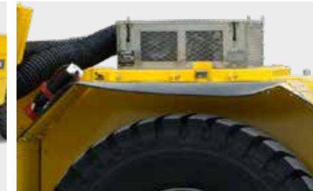
The optional air conditioning system available for the cabin provides cool air when desired and is contained with a sturdy, easy accessible box for trouble-free maintenance.
