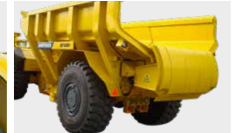
Minetruck MT436B can be equipped with a Teletram dump box, which pushes material off horizontally so it can be released in lowered areas with a low back height.
