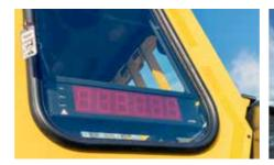
An additional load weighing display is available as option. Thanks to the additional display, the loader operator is enabled to optimize the fill factor of the dump box. This also minimizes the risk of overloading.
