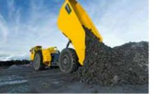
The robust dump box has a load capacity of 65 metric tonnes and the load-weighting system monitors the loading process.
