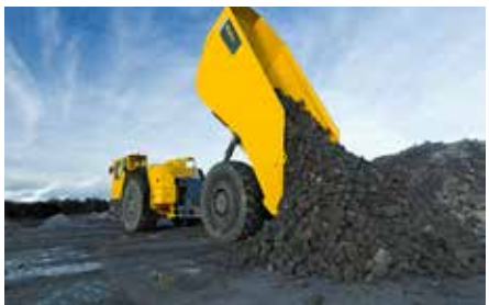
The robust dump box has a load capacity of 65 metric tonnes and the load-weighting system monitors the loading process.
