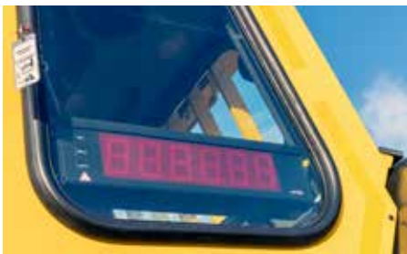
An additional load weighing display is available as option. Thanks to the additional display, the loader operator is enabled to optimize the fill factor of the dump box. This also minimizes the risk of overloading.
