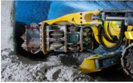
Durable steel disc cutters
