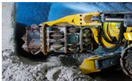
Durable steel disc cutters.
