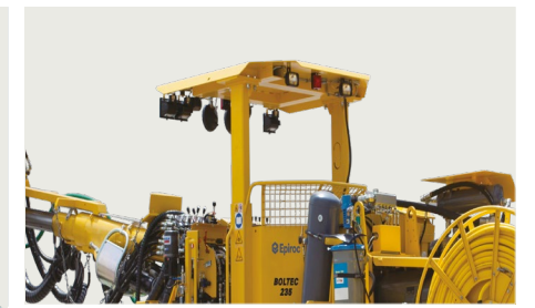
DC 15 sturdy common carrier. "Open" carrier designed for easy service to reduce down-time.
