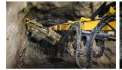
The bolting unit on the Boltec E has been optimized to reduce the overall feed length by 100 mm when compared to earlier bolting unit designs.
