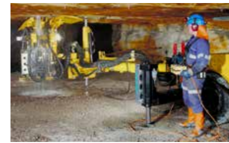
Operator panel is designed such the operator performs drilling from behind the support legs of the machine.
