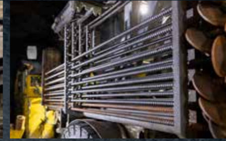
Bolt magazine with the capacity of carrying up to 44 SDA bolts.
