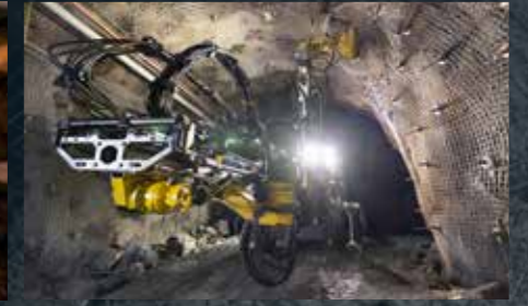
Reloading of feed magazine from the big bolt magazine.
