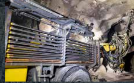
BUT 45 boom used for installing SDA and mesh.
