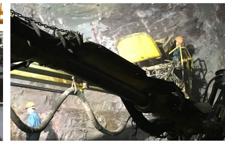
Service basket also equipped with FOPS approved protective roof, which gives the operator a safer operation environment
