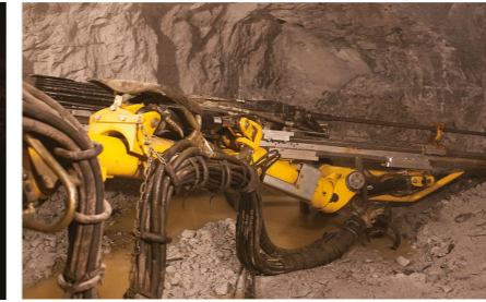
Installed with solid and robust boom BUT28. The excellent stability and accuracy of movement give fast positioning, low drill steel costs and straight holes.
