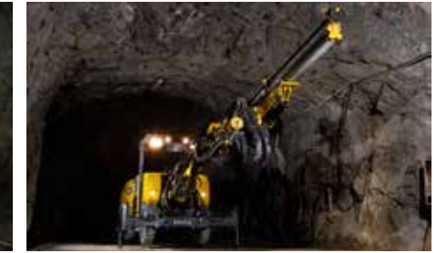
Boomer S1 can cover a large work area thanks to 70 meters of water hose and extended electrical cable.
