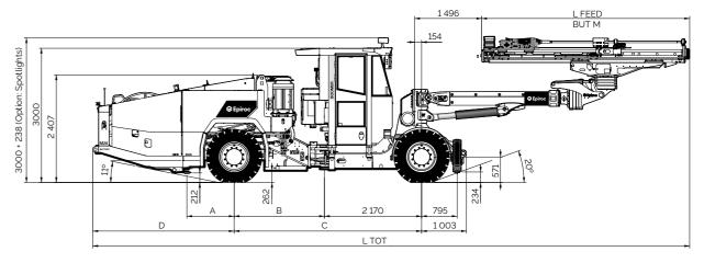
Boomer M20 Battery equipped with COP MD20.
