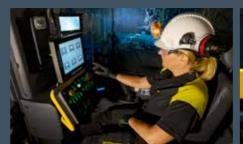
RCS-based carrier control system with logging and reporting functions means easier and faster maintenance and an enabler for tramming automation.
